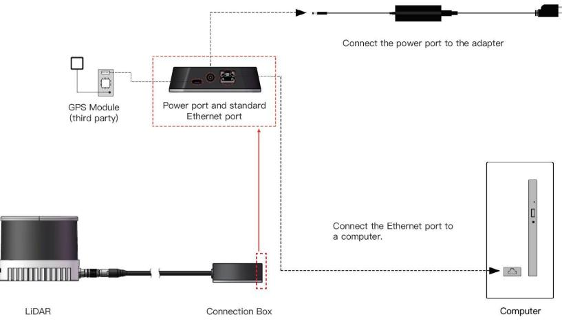
Figure 2.9 Connection Box (Connection with GPS)
