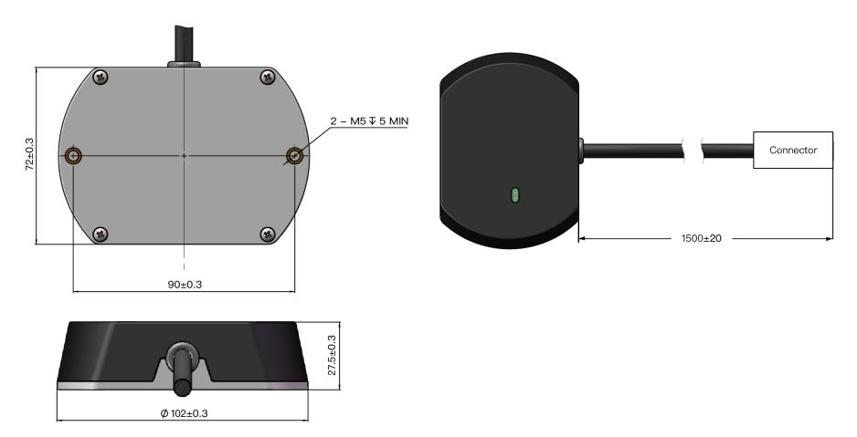
Figure 2.6 Connection Box (Unit: mm)
