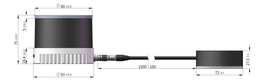
Figure 2.1 Front View (Unit: mm)
