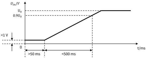
Figure IV.1 Voltage Requirements during a Power-Up
