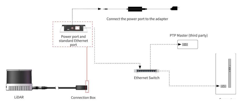
Figure 2.10 Connection Box (Connection with PTP)
