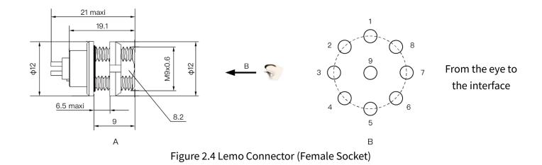
Lemo part number: EEG.0T.309.CLN (female socket, on the lidar)
