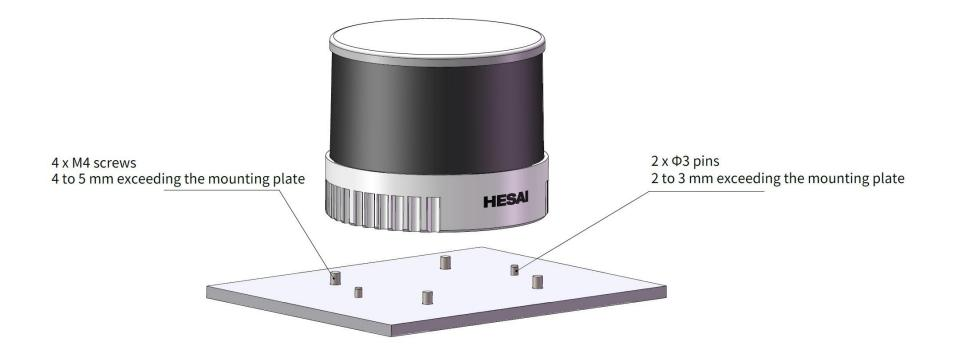
Figure 2.3 Recommended Installation
