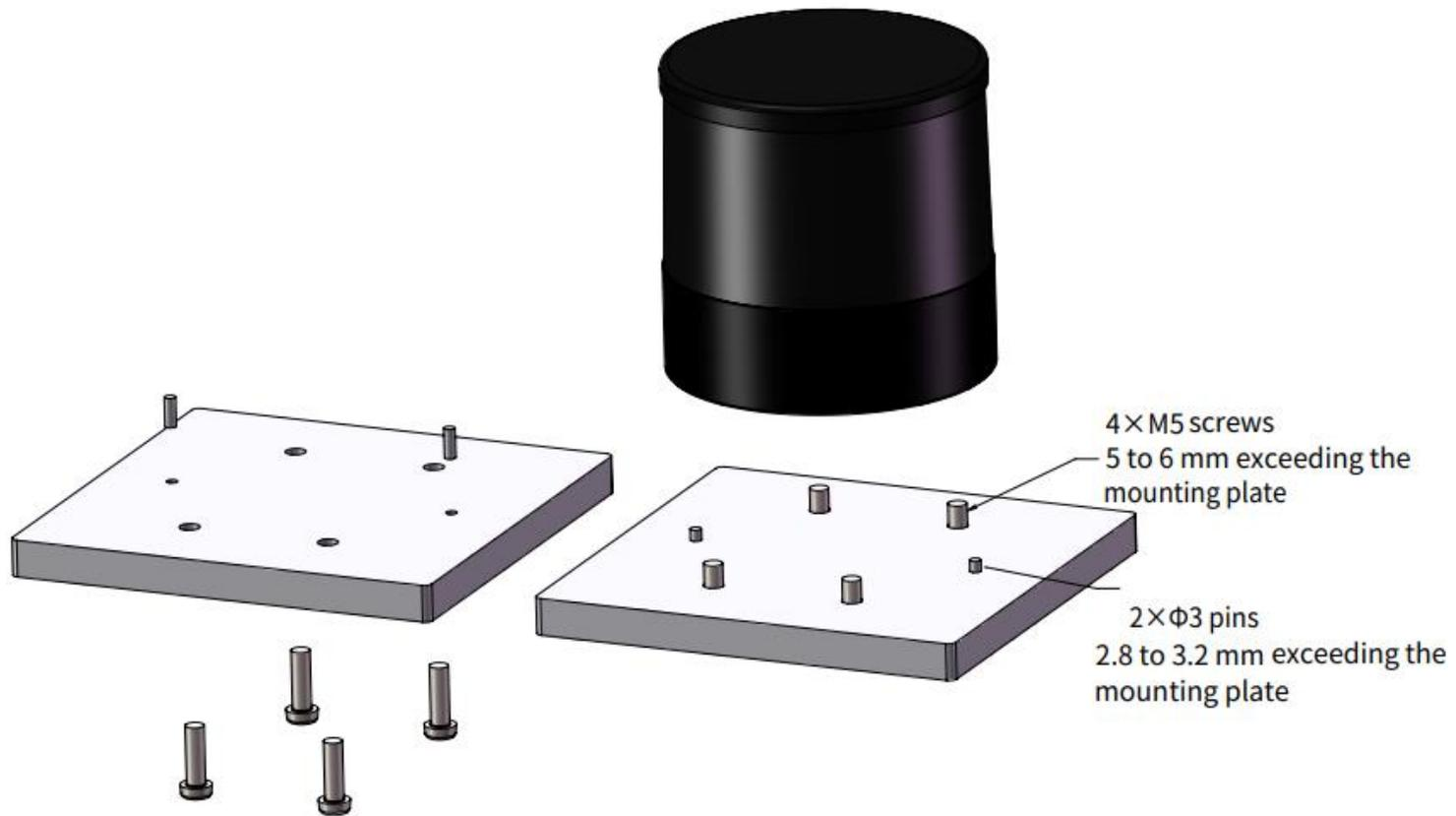
Figure 2.3 Recommended Installation
