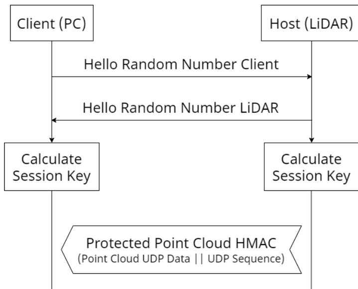
Figure 4.1 Generation of Point Cloud Signature
