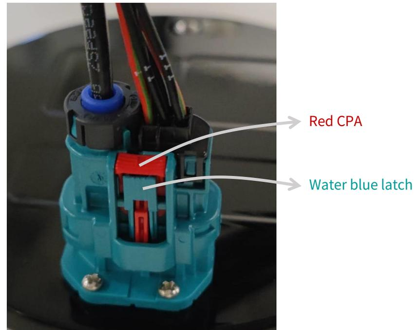
Figure 2.4 Rosenberger Connection/Disconnection
