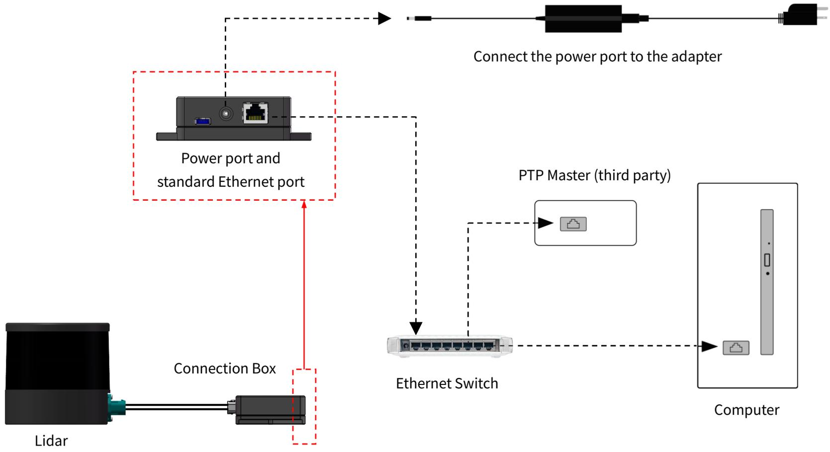
Figure 2.9 Connection with PTP (Hardware Device)
