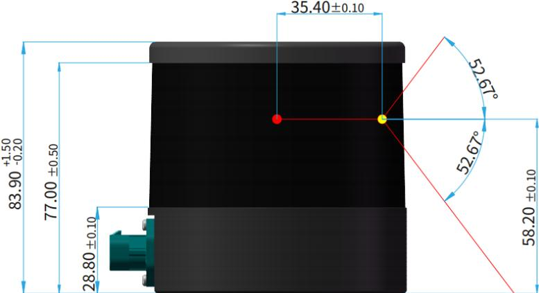
Figure 1.6 Laser Firing Position (Unit: mm)
