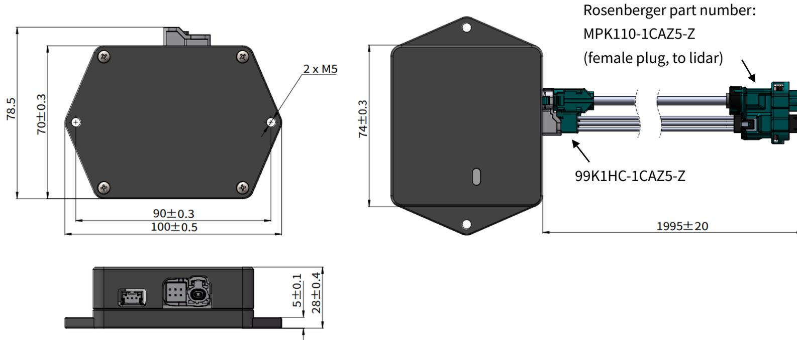
Figure 2.5 Connection Box - Connection (Unit: mm)
