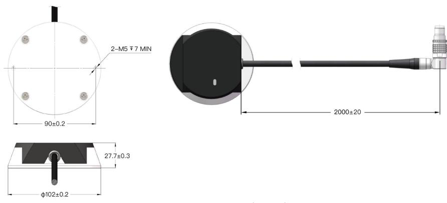
Figure 2.7 Connection Box (Unit: mm)
