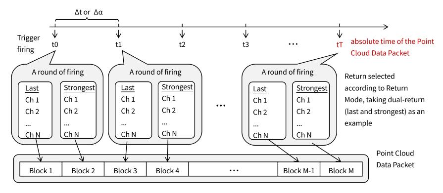
This absolute time is output to the **Date & Time** field and the **Timestamp** field in Point Cloud Data Packets.
