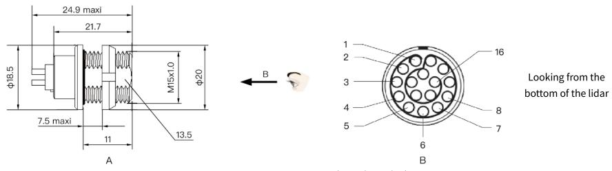
Figure 2.5 Lemo Connector (Female Socket)
