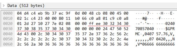
Figure 3.4 GPS Data Packet - UDP Data (Example)
