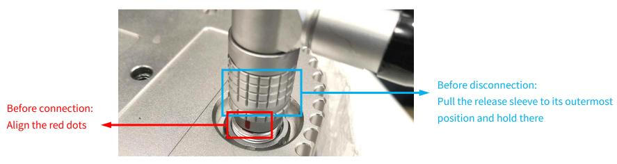
Figure 2.6 Lemo Connection/Disconnection
