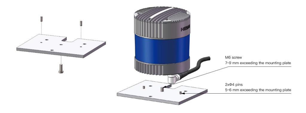
Figure 2.3 Quick Installation
