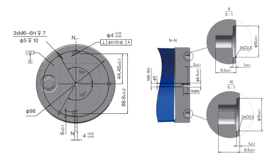
Figure 2.2 Bottom View (Unit: mm)
