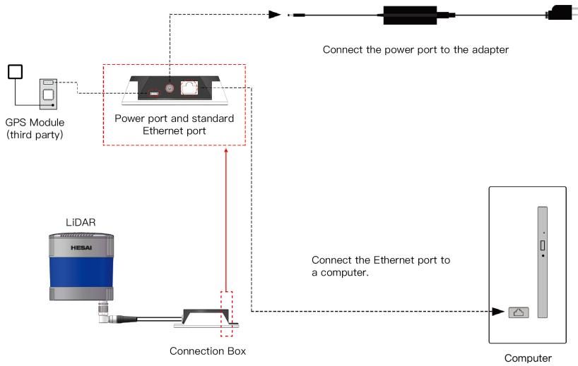
Figure 2.10 Connection with GPS
